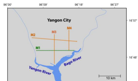
Figure 2: Map showing the MUSE seismic deployment profiles in Yangon. Orange profiles were deployed in March 2020; the green profile is yet to be deployed. The small triangles in each line represent nodal station locations.
