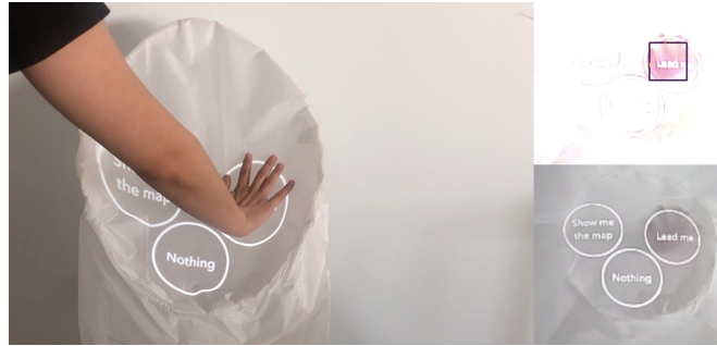
Fig. 17. A robot’s skin can be augmented into an interactive touch screen by integrating ShadowSense with a projector. Users can instruct robot by pressing the virtual buttons.
