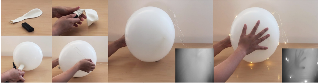
Fig. 15. Concept sketch of adding ShadowSense to a balloon. The balloon could become a touch-sensitive object, responding to touch by illuminating an LED strip.
