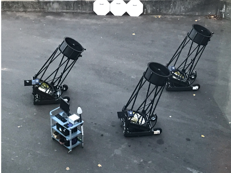
Figure 1. The Southern Connecticut Stellar Interferometer (SCSI). The detectors sit in the eyepieces of the 60 cm telescopes and are wired to different input channels of the PicoQuant correlator. (The correlator is the white box on the computer cart.)
