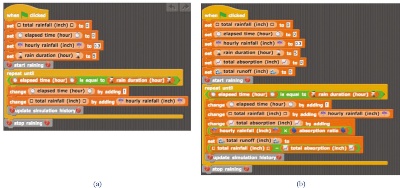
Figure 2. Computational model (a) that students began with using and (b) an example of a final computational model that students created to predict absorption and runoff for different materials.
