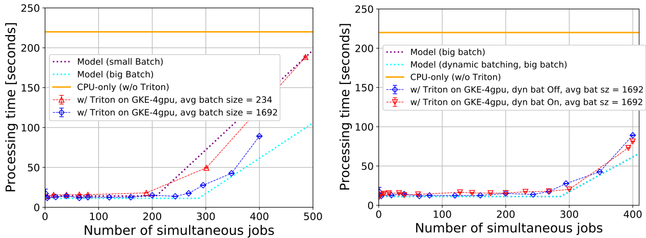
Figure 7. Processing time for the EmTrackMichellId module as a function of simultaneous CPU processes, using a Google Kubernetes 4-GPU cluster. Left: small batch size vs. large batch size, with dynamic batching turned off. Right: large batch size performance with dynamic batching turned on and off. In both plots, the dotted lines indicate the predictions of the latency model, specifically Eq. (4).
