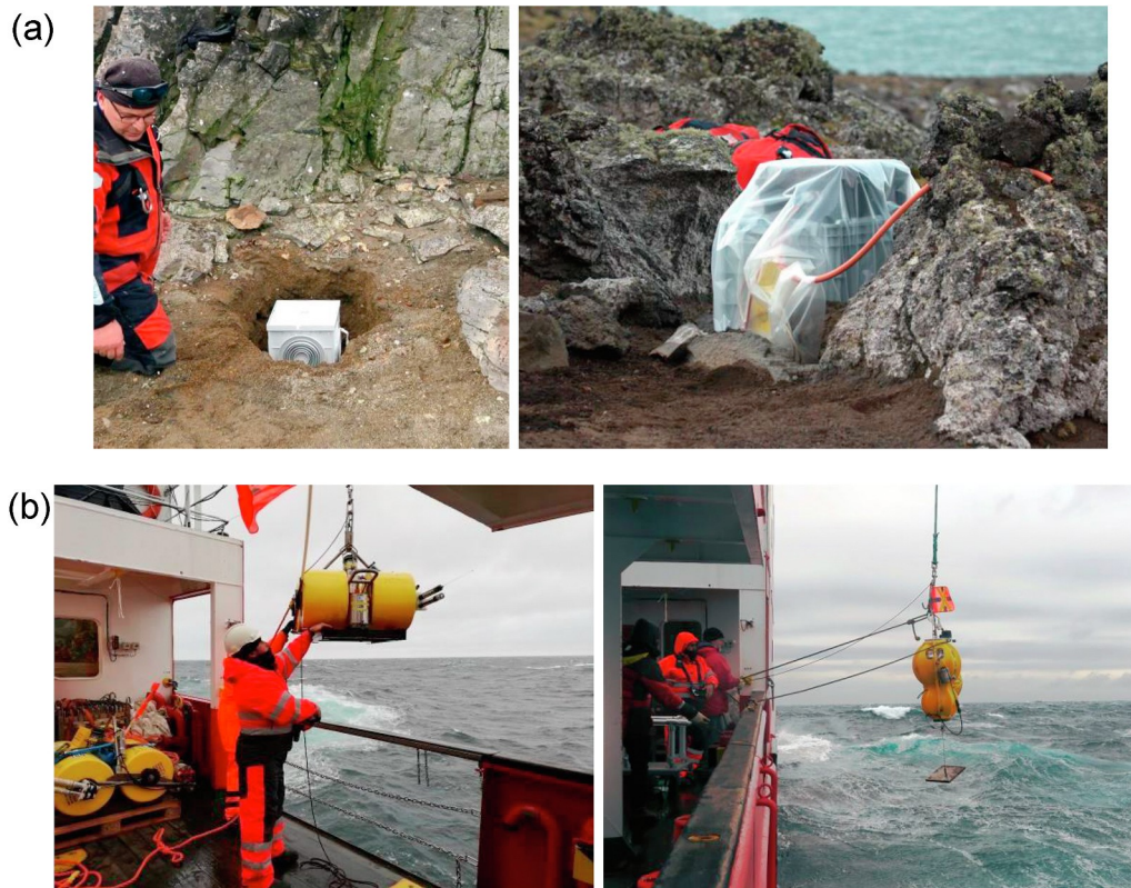
Fig. 3. (a) Installation of a land seismometer inside a buried protecting case at Snow Island (left) and final aspect of the battery pack and acquisition system (height ~0.6 m) of station PEN at Penguin Island (right). (b) Deployment of broadband (left) and short-period (right) OBS during the BRAVOSEIS 2019 cruise.
