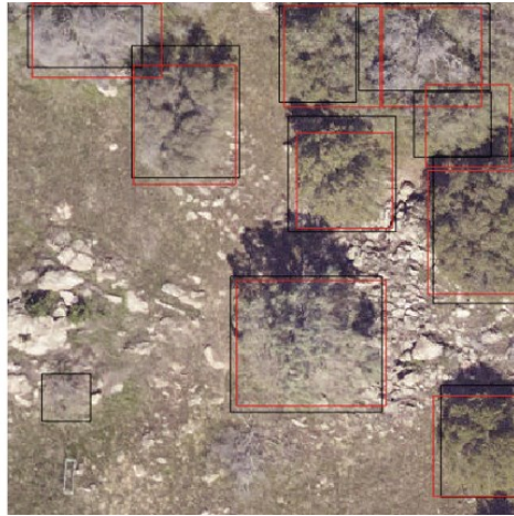
Figure 6. Example evaluation from the NeonTreeEvaluation R package. Predicted boxes (see below) in red and ground truth boxes are in black. In this image there are 10 image-annotated boxes, and 9 predictions. Each prediction matches an image-annotated box with an intersection-over-union score of greater than 0.4. This leads to a recall score of 0.9 and a precision score of 1.
