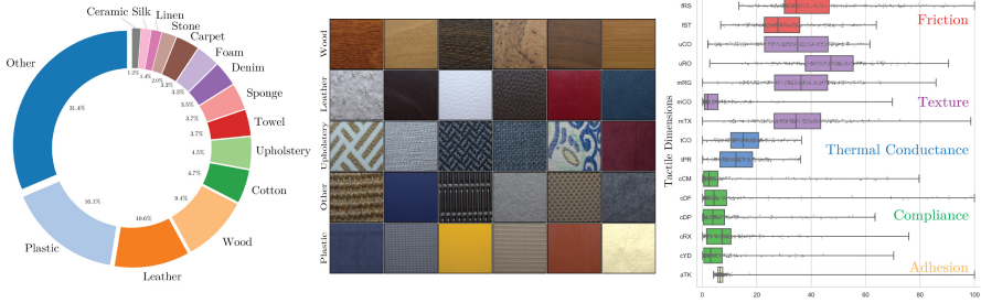
Fig. 2. Dataset statistics. Left: The distribution of material labels. The output of the models are tactile properties and not material labels. The other category includes materials with less than six occurrences. Center: A sampling of the 400+ materials in our dataset, which highlight the diversity in visual appearance. The other category includes materials such as metal, fur, corduroy, nylon, and more. Right: A box plot distribution for each tactile property. The acronym for each property is defined in Table 1.
