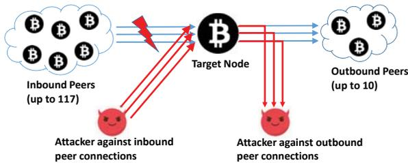
Fig. 1: Illustration of ConMan, where the target node’s *inbound* connections are initiated by the attacker and *outbound* connections are hijacked by the attacker.
