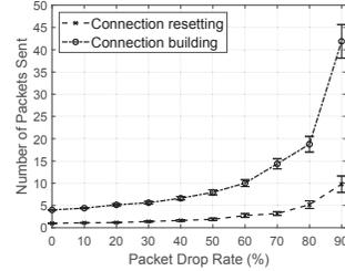
Fig. 7: The packets needed for ConMan with respect to the drop rate. The “connection resetting” (in TCP Reset) equally applies to the attacks against inbound and outbound connections, but the “connection building” only applies to the attacks against inbound connections.
