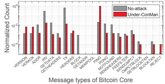
Fig. 11: Anomaly detection feature for comparing the frequency of messages ( $\Lambda$ ): the no-attack case and the under-ConMan case have the correlation coefficient  $\rho = 0.025$ .
