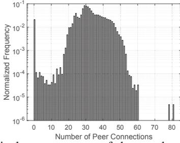
Fig. 4: Empirical measurement of the number of connections (log scale) when there are no ConMan attacks.
