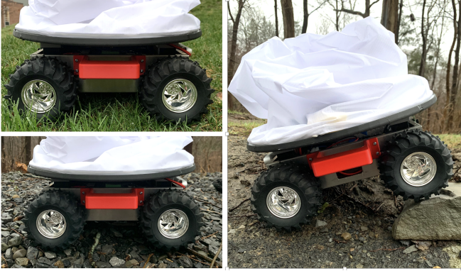
Fig. 4: The Dagu Wild Thumber gives the rover mobility over relatively rough terrain as well as conventional HRI lab spaces such as carpet and tile.
