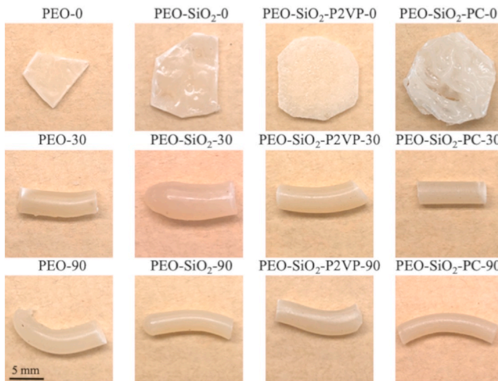
Fig. 2. Surface quality of various samples after extrusion. The top row shows unprocessed samples.
