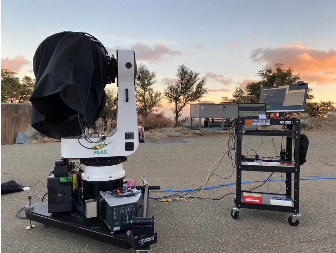
Figure 8. PEAS at Lick Observatory just before achieving first-light on 25 November 2020. The telescope and rolling pier mount are on the left, looking toward the southern skies, just east of the Shane 3-m dome on Mt. Hamilton. The computer cart at right holds the Windows machine that runs the software for the Planewave, SBIG, and Andor.
