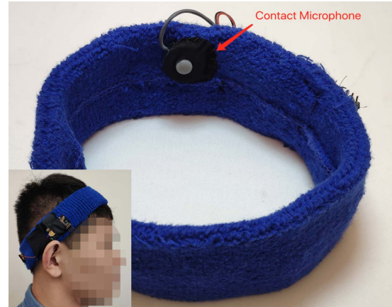
Fig. 3. Auracle prototype after our revision, using elastic headband.
