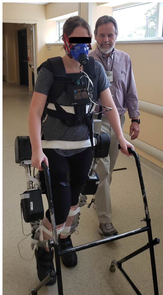
FIGURE 3 | An able-bodied pilot in the MAHNP wearing the K5 Metabolic Analyzer.
