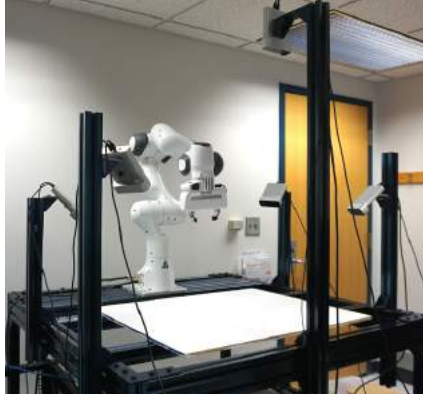
Figure 7: Experimental Setup with 5 cameras mounted around the robot arm. We combine the 3D point cloud output from each camera to create a full 3D scene.
