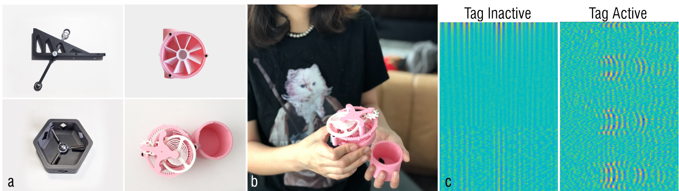
Figure 1. MechanoBeat uses (a) different electronics-free harmonic mechanical oscillator designs on everyday objects like (b) a pill bottle to automatically generate different unique mechanical heartbeat signals. At the moments of (b) user-object interaction, MechanoBeat tags generate unique mechanical heartbeats which are illustrated in the form of a radargram (c) An ultra-wideband radar array scans the living space and can reliably detect the unique mechanical heartbeat in both line-of-sight and non-line-of-sight conditions (e.g., through walls).
