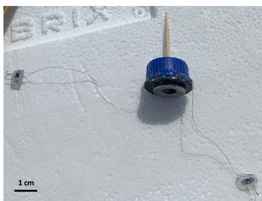
Figure 4. Side view of a two-electrode swim controller to show the flat polypropylene piece (black), with a silver washer to ballast the system. Scale bar, 1 cm.
