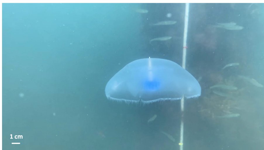
Figure 9. Representative image from in situ experiments. A biohybrid robotic jellyfish in field conditions, with the background markers (red and yellow) on the rope visible.
