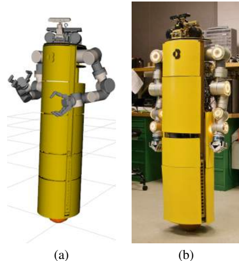
Fig. 1: The human-size CMU ballbot in (a) dynamic simulation environment and (b) dynamically balancing in reality.
