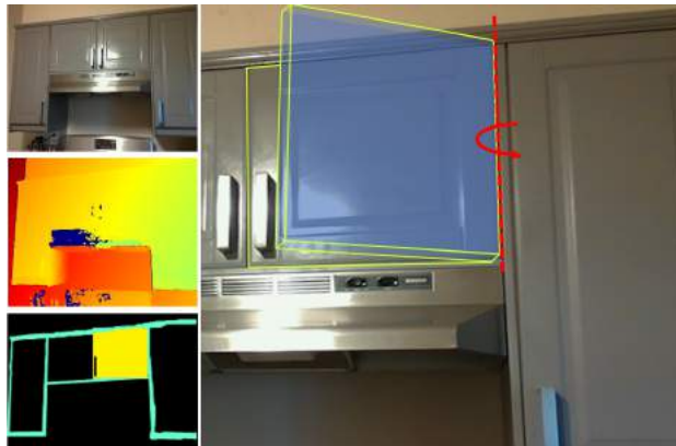
Fig. 1: Predicting articulation mechanisms using FormNet. Given the inputs on the left (RGB-D image and segmentation masks of a pair of object parts), a neural network predicts the articulation type (revolute, prismatic, fixed, or unconnected) and appropriate articulation parameters (e.g., location and direction of revolute axis). The network is trained on synthetic data and infers articulation parameters via predicting motion residual flows.
