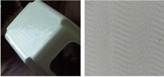
Fig. 2: Example of bi-scale material in real life. The large-scale appearance of the top of a step stool (left) that appears to have a pattern with two materials, but actually it is the same micro-BRDF with two different meso-scale geometries in the wavy pattern (right).
