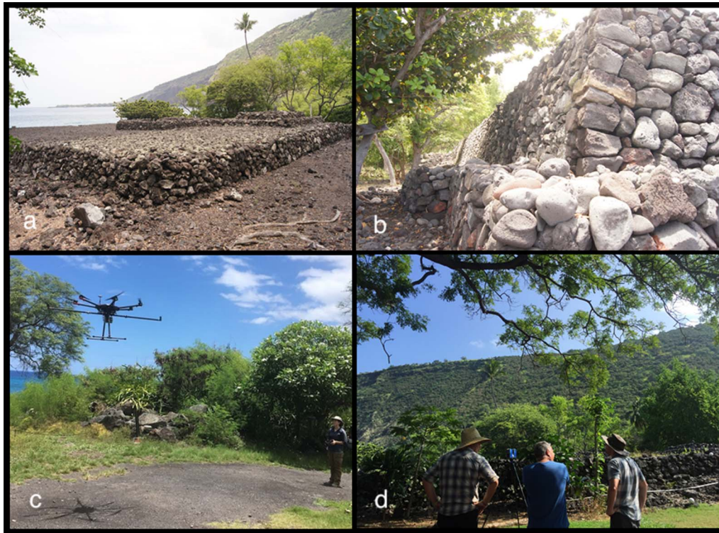
FIGURE 4. Lidar survey in Kealakekua, Hawai'i Island. Hikiau Heiau is large temple build on a natural outcrop. Much less building material was required on the (a) southeast corner compared with the (b) northwest corner. Survey using lidar mounted on a (c) UAV and (d) tripod were used to estimate the volume of building material for Hikiau Heiau and the Great Wall. (Photos by Mark D. McCoy.)
