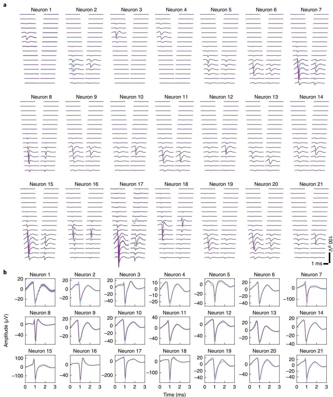
Fig. 3 | The neuron spike waveforms in different recording sessions from one mouse. a , Spatial profiles of spike waveforms of all 21 neurons recorded across 32 channels in three recording sessions marked by three different colors. Many neurons exhibit stable waveforms that are most prominent in adjacent channels. b , Spike waveforms of all 21 neurons from the channel with the largest amplitude recorded in three sessions. Different colors indicate different recording sessions, as in a . The waveforms of the same neuron recorded at different sessions are highly similar.
