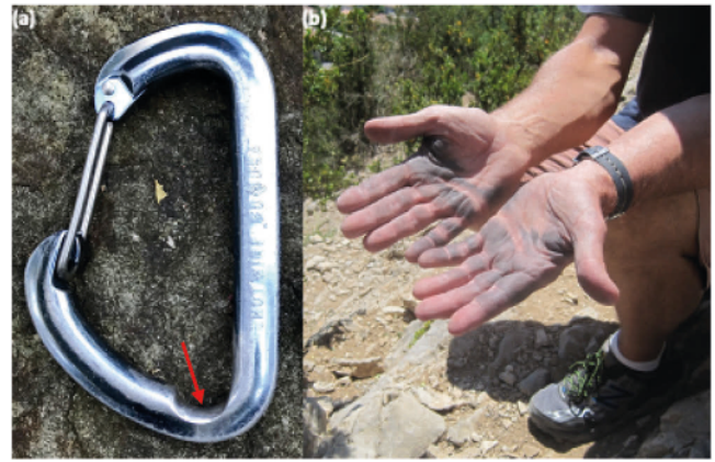
Fig. 2. (a) Abraded climbing carabiner with red arrow indicating the location of the abrasion notch, (b) Author's (HM) hands after a day of belaying and climbing. (For interpretation of the references to color in this figure legend, the reader is referred to the web version of this article.)
