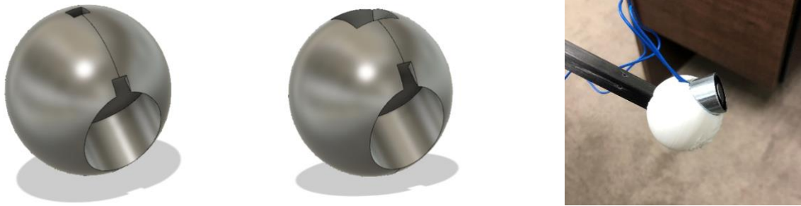
Figure 4- (a) Endpoint model for thinner-rod tensegrity (b) Endpoint model for thicker-rod tensegrity (c) Endpoint with magnet inserted
