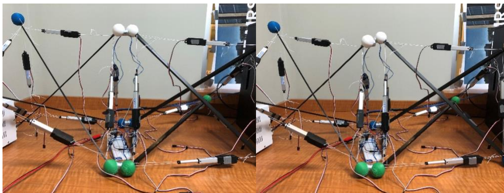
Figure 5- (a) Tensegrities connected in initial position (b) Tensegrities disconnected due to a change in a linear actuator
