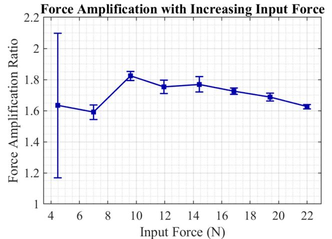
**Figure 1:** Force amplification ratio during BR tendon tensioning (3 trials, n=1).
