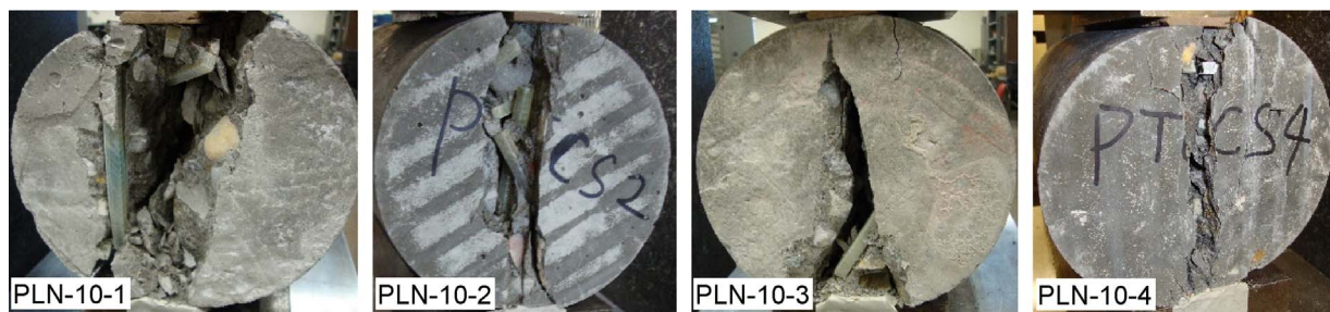
Fig. 13. PLN-10 specimens tested for splitting tensile strength after failure.
