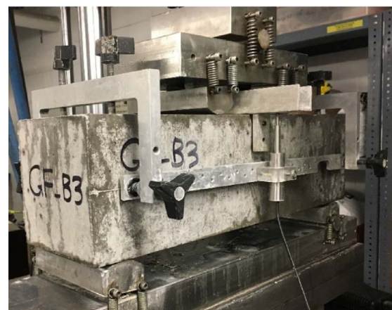
Fig. 6. Closed-loop bending test setup for measuring concrete flexural strength and toughness.
