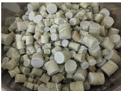
Fig. 1. FRP-RA used as a replacement of coarse aggregate in concrete.
