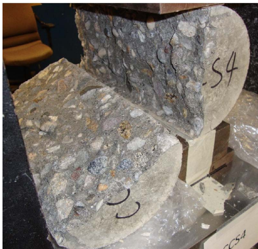
Fig. 9. A control specimen tested for splitting tensile strength after failure.
