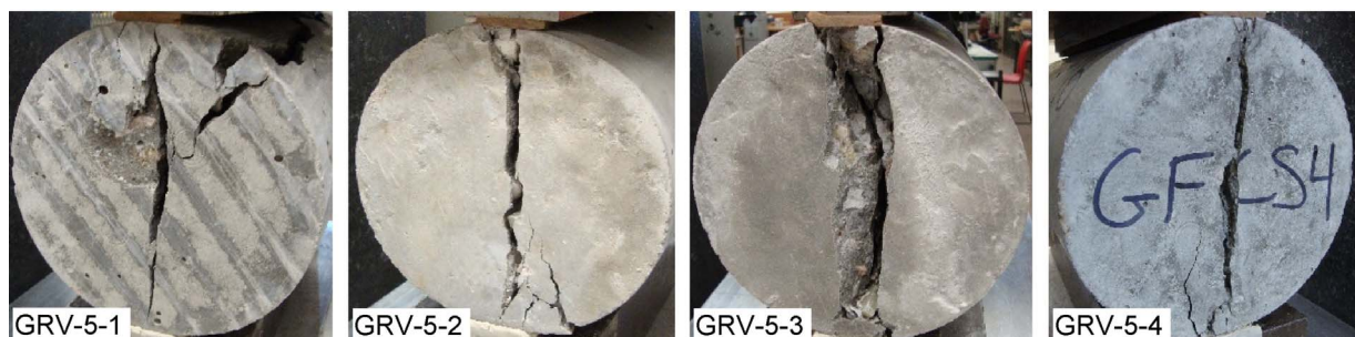
Fig. 10. GRV-5 specimens tested for splitting tensile strength after failure.
