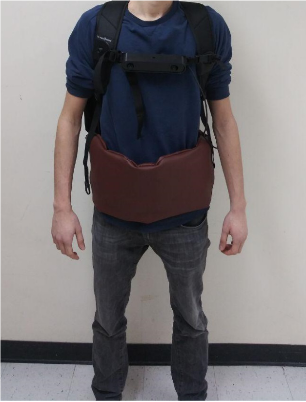
Fig. 3. Overall system on a person. The belt, here exposed for the sake of clarity, can be worn below personal garments. The camera, fixed on one of the two backpack straps, is locked in position with a buckle after the backpack is worn.
