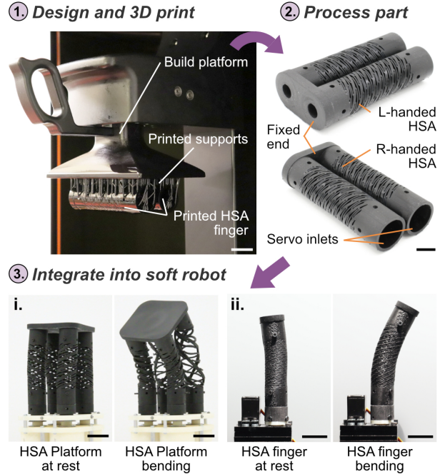
Fig. 1. A recipe for electrically-driven soft robots via 3D printed HSAs. Step 1: HSAs are designed and 3D printed via digital projection lithography. The photograph shows a complete HSA finger at the end of 3D printing. Step 2: Parts are post-processed. A final, complete HSA finger is shown. Step 3: Parts are integrated into soft robots. 3D printed HSAs are used in (i) 4-DoF, soft robotic platforms and (ii) assembled into bending actuators as HSA fingers in soft grippers. Scale bars are 25 mm, except in Step 2, where the scale bar is 10 mm.
