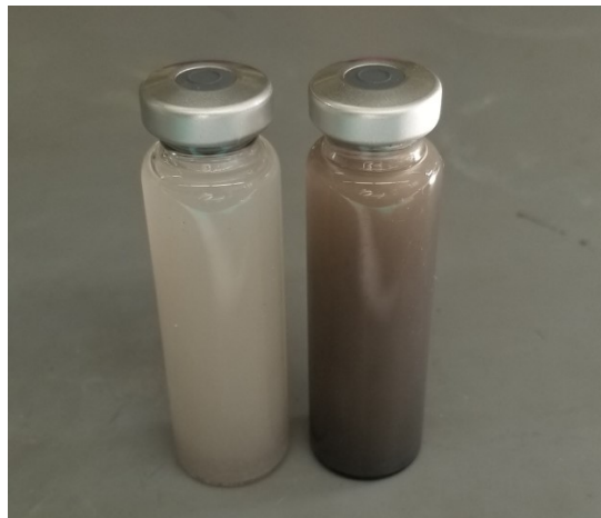
Fig. S1: H-terminated nanodiamond samples suspended in benzene solution in sealed crimp-vials. Left: air-annealed prior to H-termination. Right: sample was not air-annealed.
