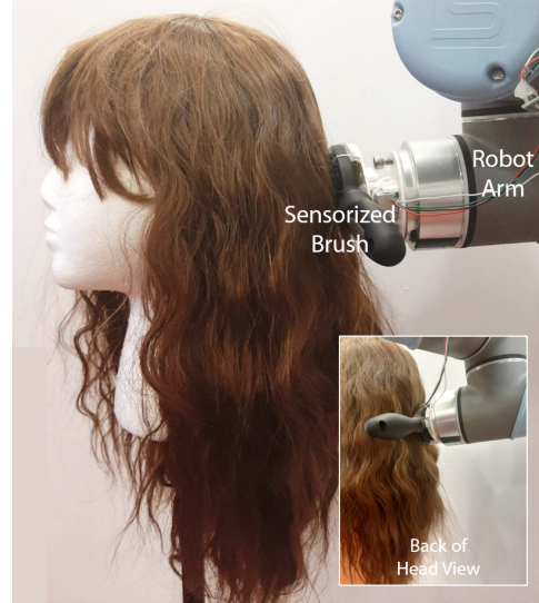
Fig. 1. Experimental setup for the investigation of robotic hair brushing showing the wig, sensorized brush and robot arm.
