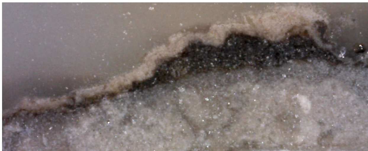
Fig. 1. Cross-section of a black paint sample (1 and 1') from Eagle Cave. For scale, the width of the section shown is \sim 0.5 cm. The black paint layer varies from 50 to 250 \mu\text{m} and consists of manganese mineral pigment, calcite, whewellite, and gypsum. Overlying the paint is a cream-colored whewellite, calcite, and gypsum mineral accretion. Underlying the paint is a grey layer of calcite and whewellite. The rock substrate is a dolomitic limestone. Mineral identifications were determined using X-ray diffraction (Steelman et al., 2021).
