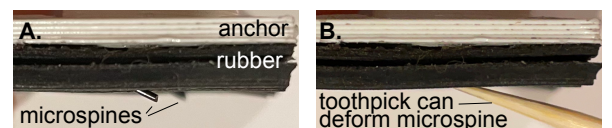
Fig. 4. A) Side view of microspine-rubber composite in flat sample. B) A toothpick is strong enough to deform a flexible microspine into the surface of the rubber.
