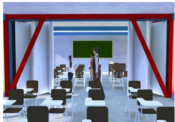
Fig. 8 Architectural Render of Classroom with Lateral Load Reinforcement
