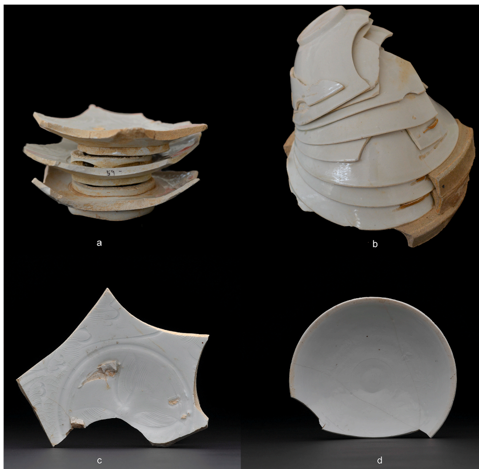
Fig. 2. Two different stacking techniques and examples of Dehua porcelains analyzed in this research. (a) The pronged-ring stacking technique. (b) The invert stacking technique. (c) Qingbai/white porcelain plate with five-prong marks (fired using the pronged-ring stacking technique). (d) Qingbai/white porcelain bowl with an unglazed rim (fired using the invert stacking technique).
