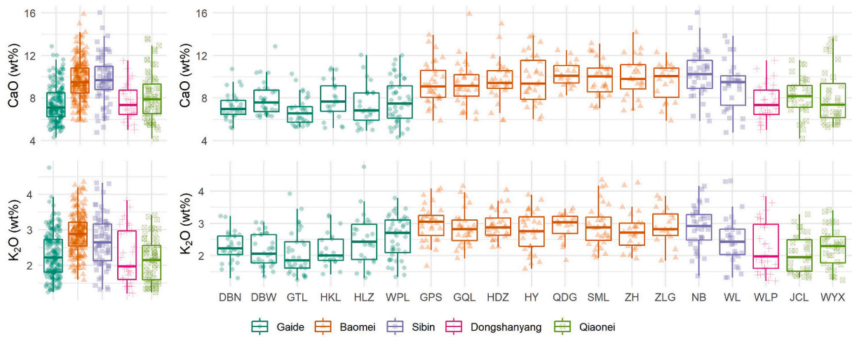
Fig. 13. Boxplots of the concentrations of CaO and K 2 O measured by pXRF for each village and each kiln.
