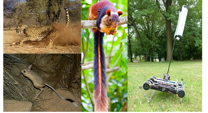
Fig. 1. Examples of biological and robotic systems with long aerodynamic tails. The cheetah, the giant Indian squirrel, and the jerboa have tails ranging from 75% to nearly 200% of their body length, motivating the aerodynamic tail presented here. Top left: Cheetah ( Acinonyx jubatus ). Bottom left: Greater Egyptian jerboa ( Jaculus orientalis ), photo credit: Elias Neideck/CC BY-SA 3.0. Middle: Giant Indian squirrel ( Ratufa indica ), photo credit: VinodBhattu/CC BY-SA 4.0. Right: The Ghost Robotics Minitaur [21], equipped with a 2x body length aerodynamic tail.
