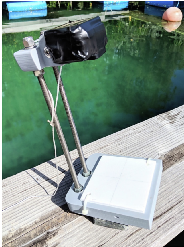
Fig. 3. CoralCam unit prior to test deployment on a CRMP platform. Before deployment a coral fragment is fixed to the center of the settlement tile. CoralCam's underwater housing is wrapped in electrical tape to limit biofouling damage – the lens is left exposed. CoralCam and CRMP were anchored to the seafloor with a dive weight in this test.
