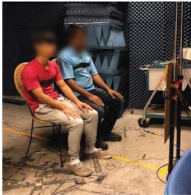
Fig. 1. Presence of multiple subjects in front of quadrature radar transceiver system in a millimeter wave anechoic chamber. A combined mixture of reflected signals returned to the radar from two subjects.
