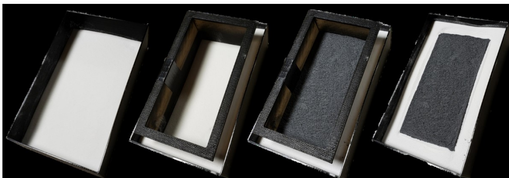
Figure 6 Process showing how the PLA forms were used to separate doped powder from virgin. a) The chamber was filled with a base layer of virgin powder. b) The form was placed in the center of the chamber and surrounded by additional powder to create a cavity. c) The cavity was filled with graphite-doped powder. d) The form was removed to create an interface between doped and virgin powder.
