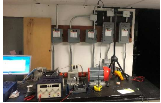
Fig. 9. Experimental Set-Up of HR-SRM
