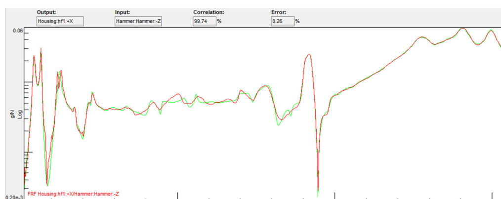
Figure 9. Experimental Frequency Response Function vs Curve Fitting for NVH testing.
