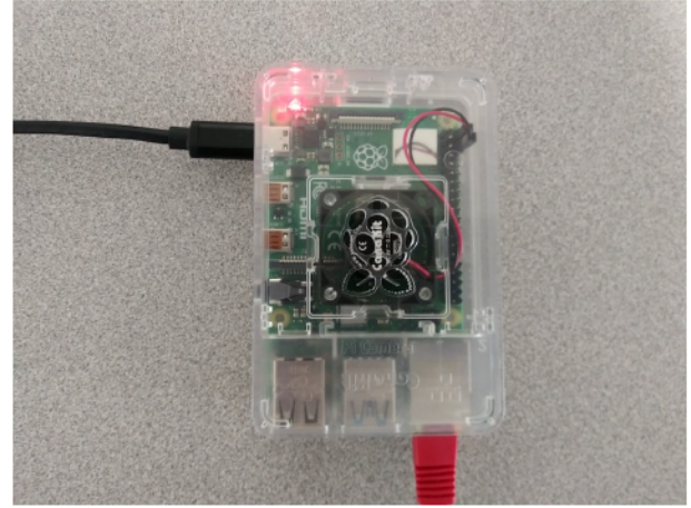
Fig. 2. Block-Pi uses Raspberry Pi 4 to setup the external network with its Ethernet port and to host the access point with its wireless interface
