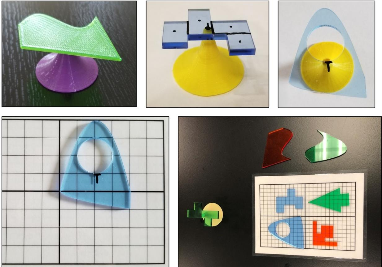
**Figure 5.** Example lamina shapes for 2D centroid activities.
