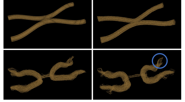
Fig. 12. Splitting and reconnection of quasi-parallel vortex tubes with vortex filament methods showing frames 1, 100, 300, and 400.
