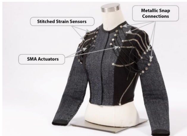
Figure 3. Generation 1: Sensing and SMA-Actuation Garment
