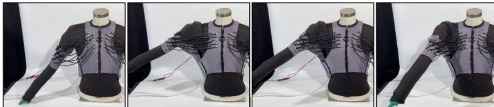
Figure 5. Actuation steps: (from left to right) (1) fully deactivated actuators, (2) partial bladder actuation, (3) partial bladder and SMA actuation, and (4) partial bladder and full SMA actuation
