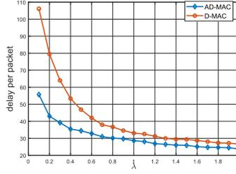
Figure 3. A comparison of the delays experienced per packet delivered over some time duration.
