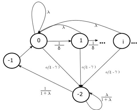
Figure 1. State space model for the Markov chain
