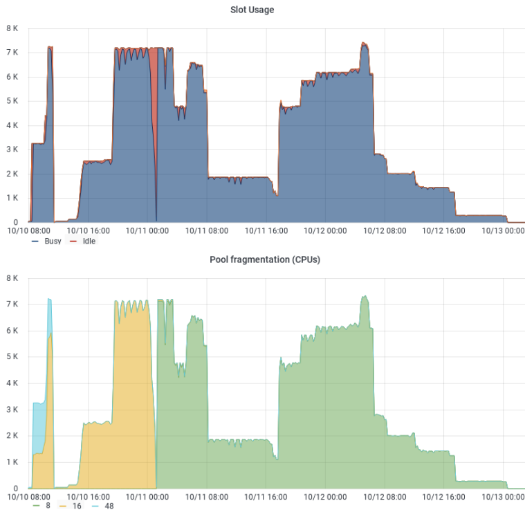
Figure 2. HTCondor split-starter model being tested as prototype for BSC exploitation: total number of CPU cores allocated to CMS during the execution of the tests, in idle or busy states (top), and total number of CPU cores employed by running jobs, successively configured to run as 48, 16 and 8-core tasks (bottom). Excellent resource utilization is observed in the three cases.
