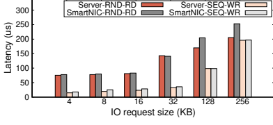
Figure 2: Read/write latency comparison between SmartNIC and Server JBOFs.
