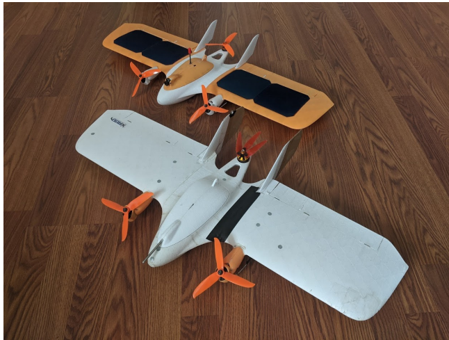
Fig. 13. Flight-Test Vehicle (front) and Solar Prototype (rear). Note the enlarged vertical stabilizer surfaces and strakes added on the Flight-Test vehicle to improve directional stability. The Flight-Test vehicle also features a folding rear propeller for improved forward flight drag.
