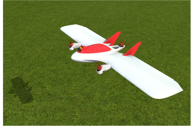
Fig. 11. RealFlight 9.5 Vehicle Model. ArduPlane SITL is used to drive the inputs to the RealFlight simulated vehicle, with the physics simulation incorporating the derived dynamics of the vehicle. Screenshot taken from [22].
