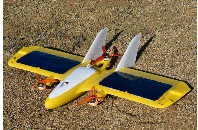
Fig. 1. Solar-Wing variant of the MiniHawk-VTOL. The wing top surface is excavated for the conformal integration of the Maxeon™ solar cell series, including wiring conduit tunnels (hidden).
