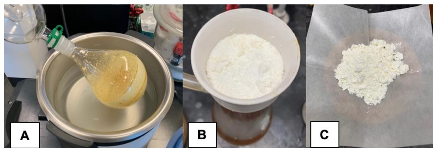
Figure 7. NCMPL product isolation: A) Crude solid following thorough removal of volatiles by rotary evaporation. B) Product after washing with methanol under gentle vacuum filtration in a Büchner funnel. C) Appearance of \gamma -lactam ( 5 ) as a powdery crystalline solid (photos provided by submitters).
