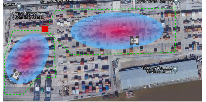
Fig. 1: Information gathering from port infrastructure monitoring: Two mobile robots gather information from blue elliptical locations within two critical regions (dotted green lines) of the Port of New Orleans, LA, USA, starting from the red depot location.
